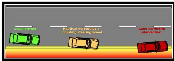
Figure 9: LDWS warns the driver if he unintentionally drifts out of his intended lane
